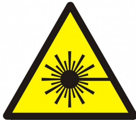
Figure 2: Laser Radiation Hazard Safety Symbol (ANSI Z535)
