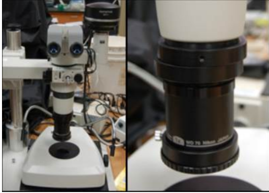
Figure 3: Nikon SMZ 1000 stereo microscope with 1x objective and dark-field polarization.
